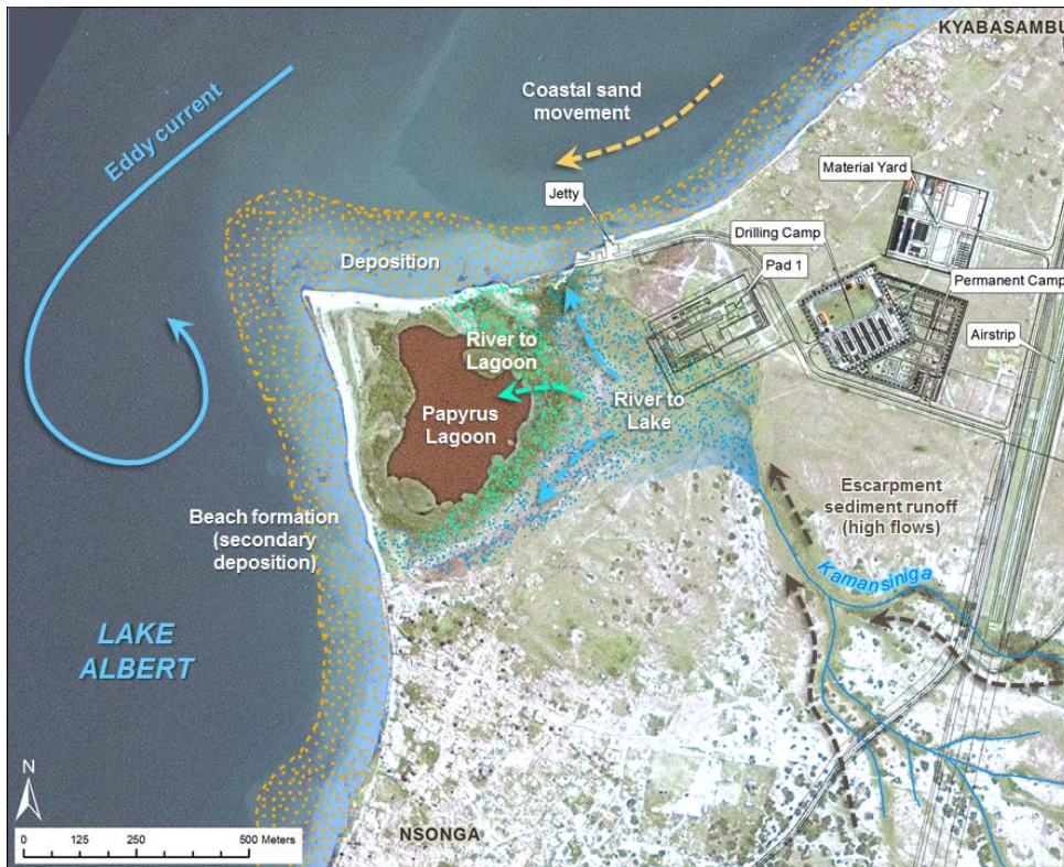
Figure 34: Likely drainage path to the Papyrus Lagoon
