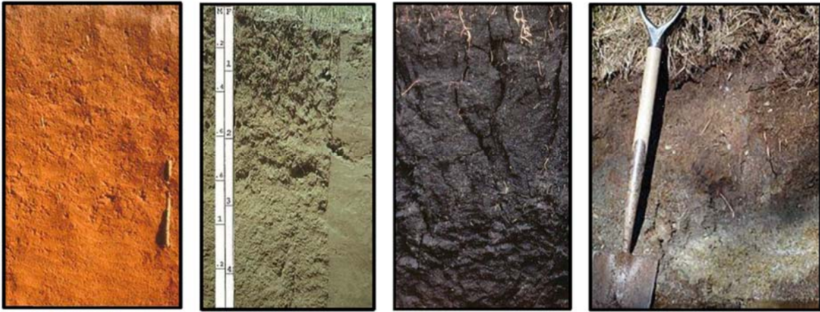
Figure 1: Examples of FAO classified soils (from left to right) - Ferralsol, Lithosol, Vertisol and Gleysol.
