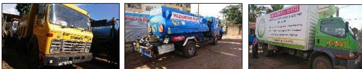
Figure 5: Examples of Modified Dump Truck (left), Vacuum Tanker (centre) and Box-body Truck (right)
