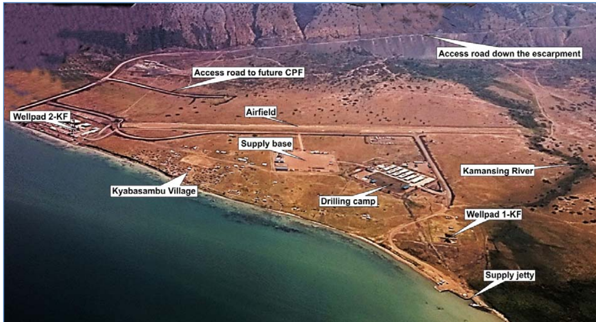
Figure 2-2: Overview of the existing main project infrastructure
