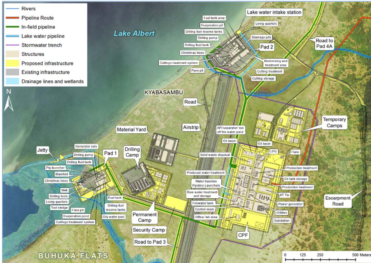
Figure 2-20: Footprint and typical layout of the CPF, showing the context of the well pads and associated infrastructure
