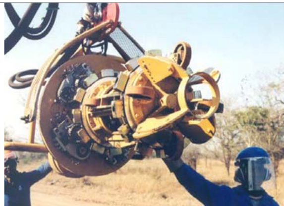
Bevelling machine for trimming pipe ends
