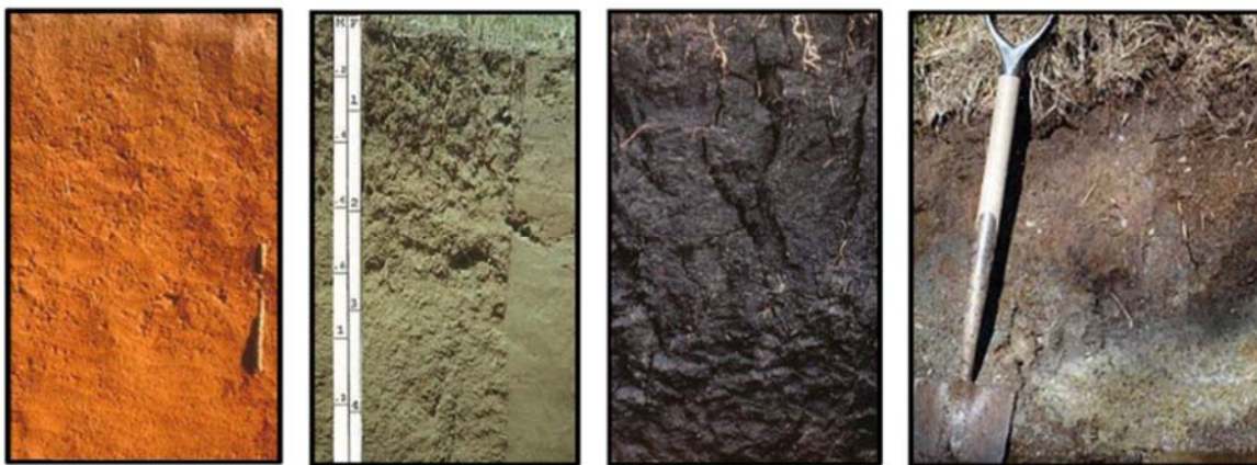
Figure 6-15: Examples of FAO classified soils (from left to right) - Ferrasols, Litosols, Vertisols and Gleysols
