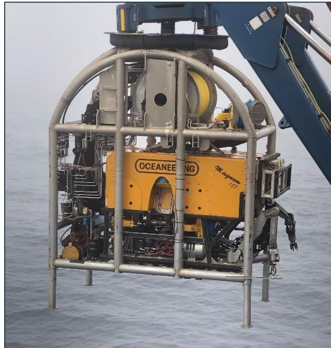
Figure 2-2 Oceaneering Magnum 157 ROV used for the Flemish Pass benthic survey in its cradle
