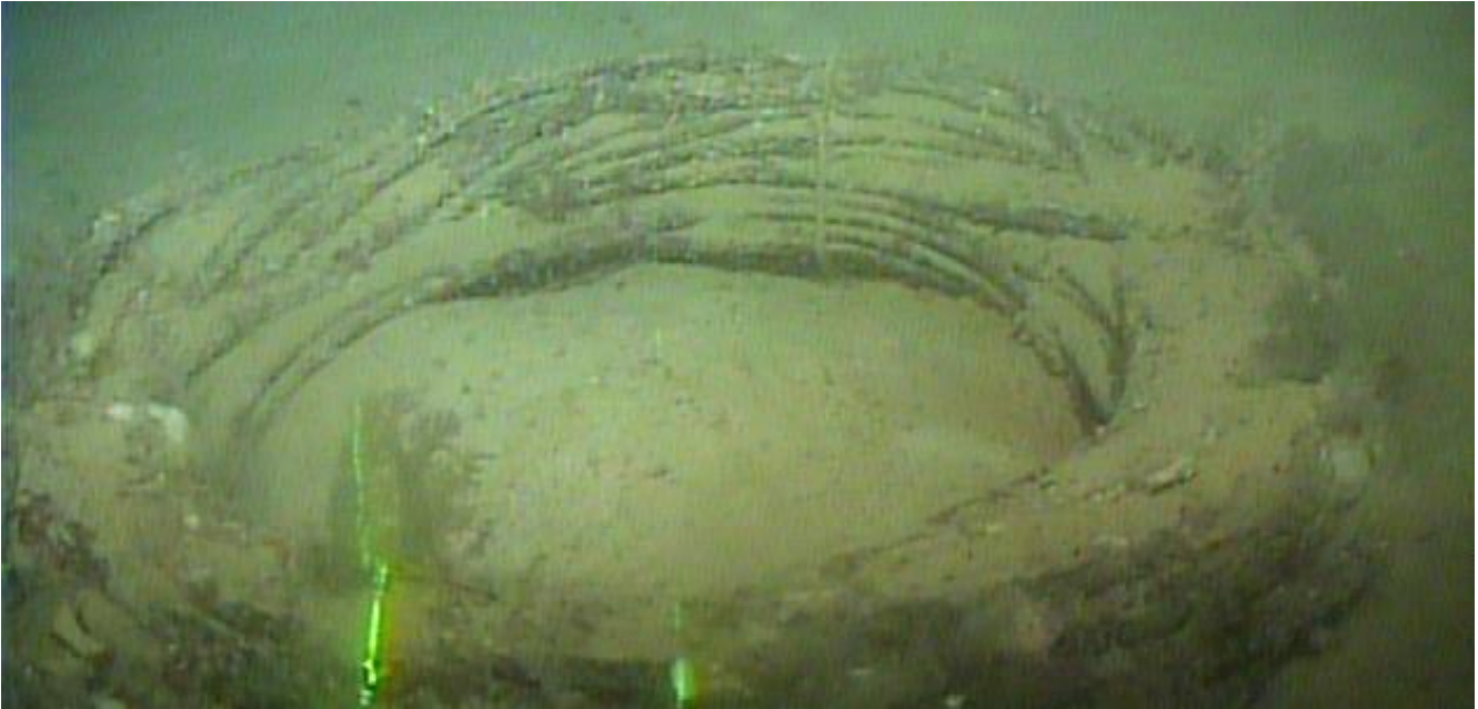
Figure 3-5 Coil of metal wire observed along Grid Line 8 at Black Knight L-91. Green lasers are spaced 25 cm apart.
