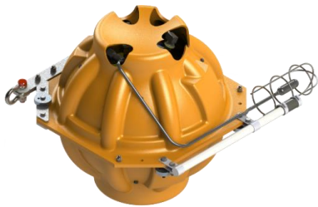
Figure 6. Autonomous Multichannel Acoustic Recorder-Generation 4 Ultra Deep (AMAR G4 UD; JASCO) used to measure underwater sound in the Flemish Pass.
