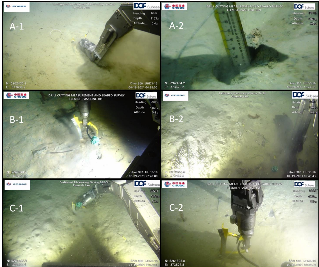
Figure 3-6 Examples of depth penetrations tests conducted within the grid lines area (A-1 and A-2), the transect area (B-1 and B-2), and a reference station (C-1 and C-2). Images on the left represent the pre-drilling depth penetrations, and images on the right are from the post-drilling survey.
