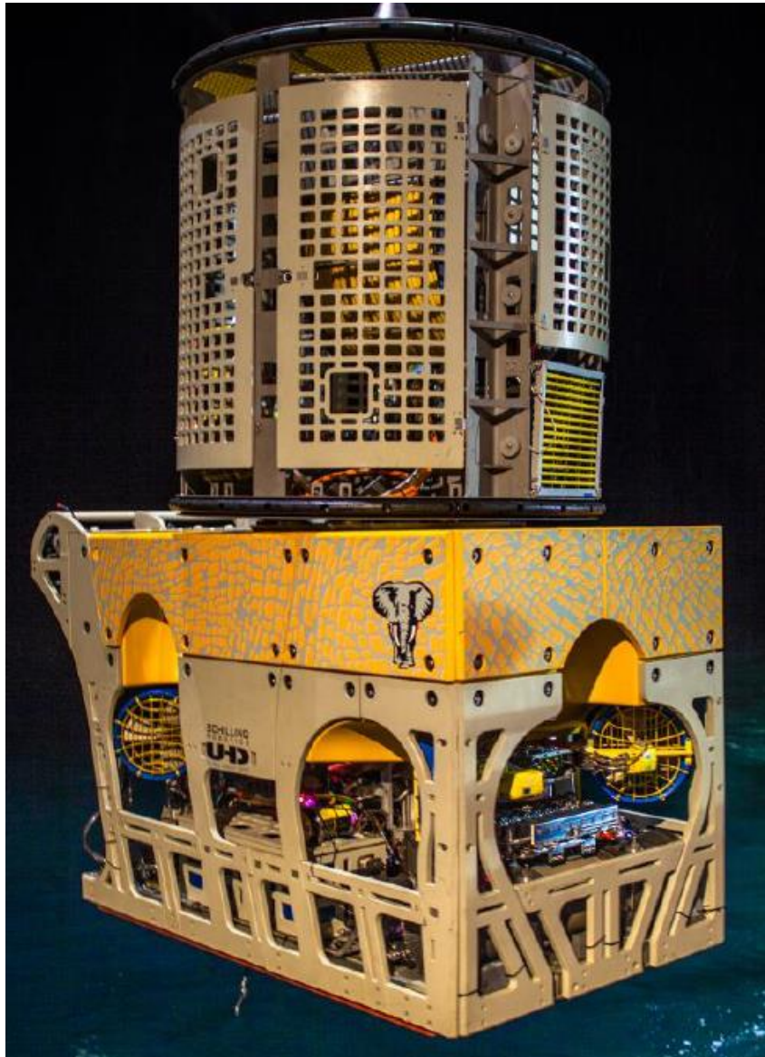
Figure 2-2 DOF Schilling ROV used for the seabed survey (Image courtesy of TechnipFMC, https://www.technipfmc.com/media/5b4p2j2r/data-sheet-schilling-uhd-iii.pdf ).
