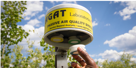
Environmental Engineer changes out a filter at a passive air station
