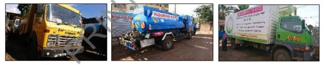
Figure 5: Examples of Modified Dump Truck (left), Vacuum Tanker (centre) and Box-body Truck (right)
