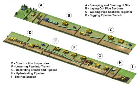
Figure 2: Construction stages of an export pipeline [Source: Association of Oil Pipelines (AOPL)]
