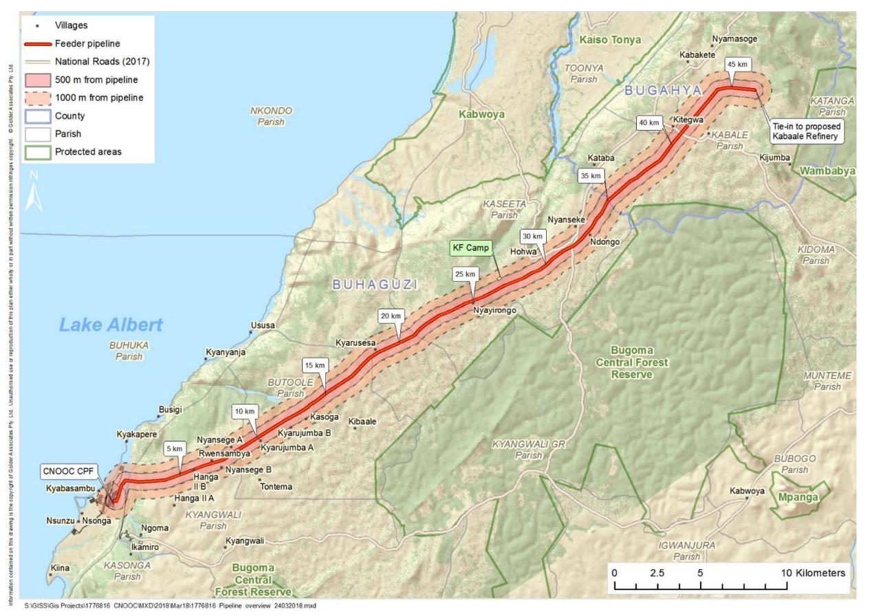
Figure 1: Location of the Feeder Pipeline (also known as the Export Pipeline).
