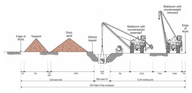
Figure 3: Schematic diagram showing the construction train for a flowline. The construction right of way width does not need to exceed 30 m
