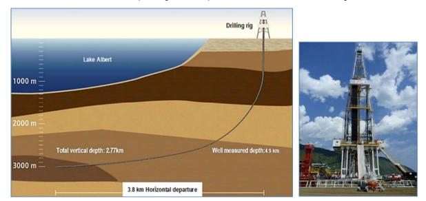
Figure 2-3: An illustration of directional drilling under Lake Albert
