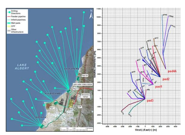
Figure 2-2: Approximate subsurface extent of the wells and wellbores (left side) with the latest extent indicated on the right as of September 2018.
