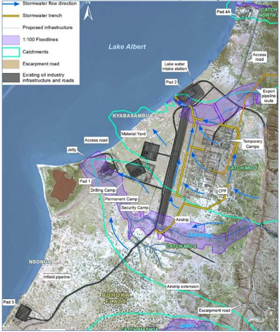
Figure 7-2: Direction of stormwater drainage from the production facility on the Flats. During construction, stormwater will carry sedimentation from earthworks and during operation, an increased risk of sediment into Lake Albert will be caused by erosion of drainage
