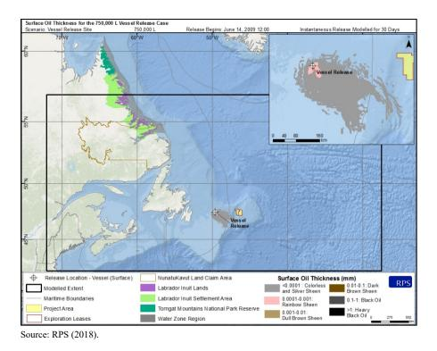
Figure 6-2. Surface oil thickness resulting from the release of 750,000 L marine diesel during the vessel collision scenario.
